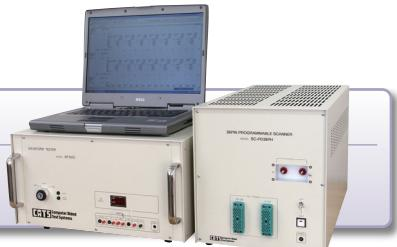
●WF3000 is waveform test system which is designed to measure reverse breakdown voltage of IGBT and leak current of 3000V. Measurement head on the picture is the combination with 36 pin programmable scanner. It can correspond to demanded measurement head.
