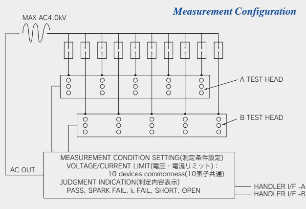
●TARY4000 is the corresponded model to multi-device of TAC series. It can measure 10 devices simultaneously to improve productivity.
