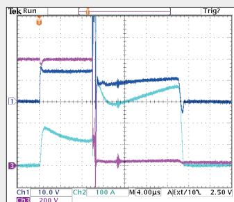
●SCT1010ZZ has been designed to test energy tolerance of IGBT device at short circuit. Energy amount is calculated by digital oscilloscope waveform which is corresponded with software. Also, it has preventive function not to break D.U.T for safety.
