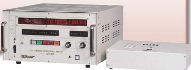
● LDV-02B is power up model that IF forcing became 2A. Power time is 9,990sec, VF measurement is 32,000mV at maximum with 1mV resolution. Moreover, it can connect to scanner such as 10 elements or 30 elements type.
