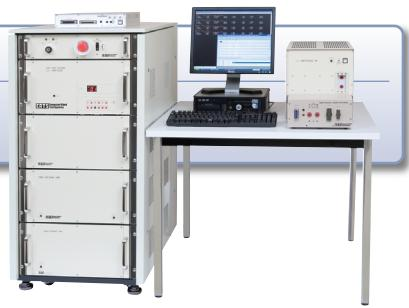
●IGBT7530Z is IGBT tester which forces high voltage of 7.5kV. This tester contains know how to measure stably such as how to decrease to occur sparking because of high voltage.
