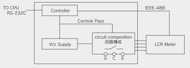
●CPS900 has been designed to measure capacitance of MOS-FETs and IGBT. Capacitance meter is not our product, however, it is controlled as one of the measurement system with tester by software.
